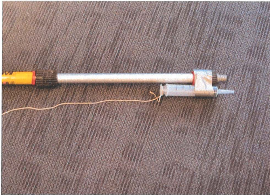
Fig 1 - Syringe Sampling Setup
